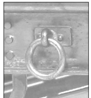
flush with the solebar back. You should now have separate moving lashing rings to secure a wagon load too and impress your friends.
